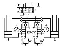
Fig. 2. Basic hydraulic diagram of props from a shield of a powered roof support
