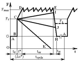
Fig. 3. The operation of hydraulic props
